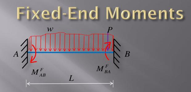
The moments at the walls or fixed joints of a loaded member are called *fixed-end-moments*. These moments can be determined from the table provided, depending
