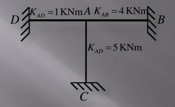
If several members are fixed connected to a joint and each of their far ends is fixed, then by the principle of superposition, the total stiffness factor at the joint is the sum of the member stiffness factors at the joint i.e.
