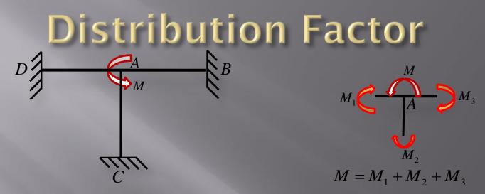
If a moment *M* is applied to a fixed connected joint, the connecting members will each supply a portion of the resisting moment necessary to satisfy moment equilibrium at the joint.
