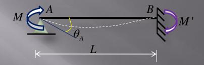
The moment *M* at the pin induces a moment of M' = M/2 at the fixed end. The carry over factor represents the fraction of M that is carried over from the pin to the fixed end. Hence, in the case of a beam with far end fixed , the carry over factor is +1/2. The plus sign indicates both the moments act in the same direction.
